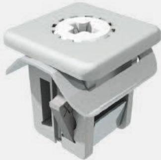
For joining of flat metal sheets acc. to Machinery Directive 2006/42EC (captive connection of locking devices). Operation by Phillips H2.
